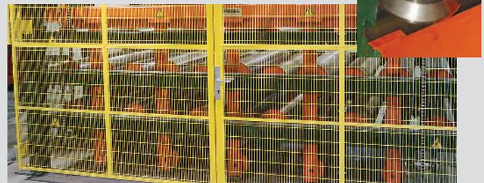
The machine frame is fabricated from high-quality square steel tubing for maximum stability and both active and passive guarding is utilized to protect the operator.
