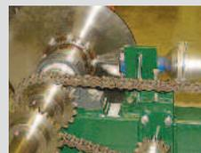
A pneumatic safety disk brake engages in the event of a chain break or if the maximum lifting or lowering speed of the carriage is exceeded.
