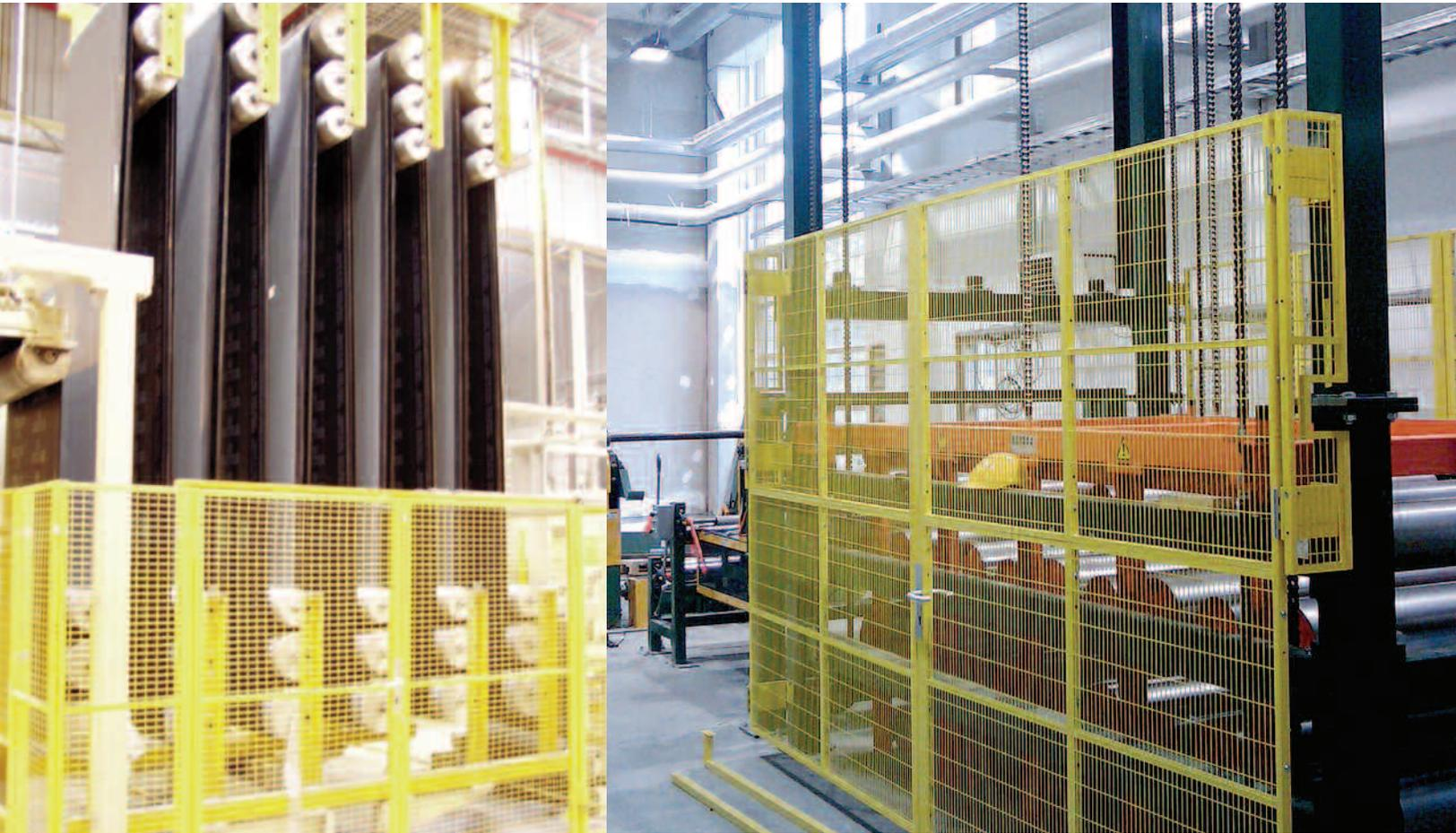
The all new **Reichel & Drews NA3000** nested accumulator can be used both as a splice accumulator for reinforcement and as a finished product accumulator.
